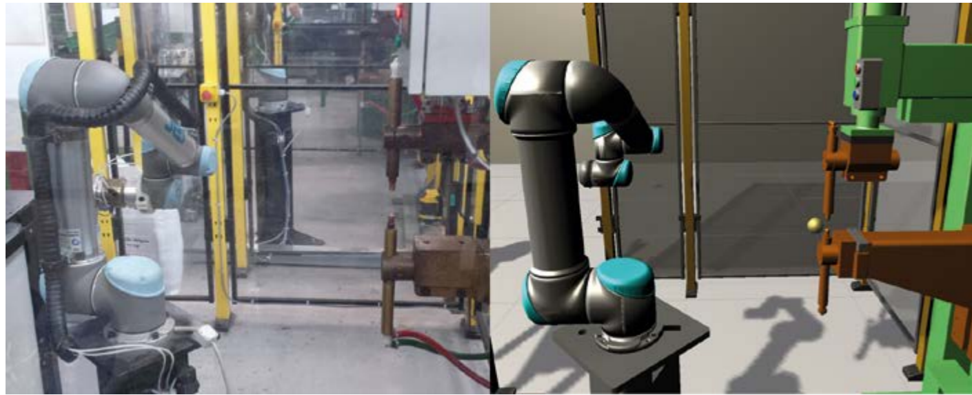
CSI: Cobot industrial case study robot cell and a representation of this in the digital twinning environment
